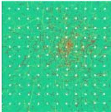
Figure 3: 10 TeV proton shower falls on near the center of the array; only charged particles are shown
